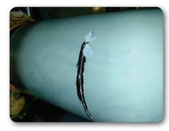
Photos (Top to bottom): Coke Conveyor, Damage on a superclendar roll
