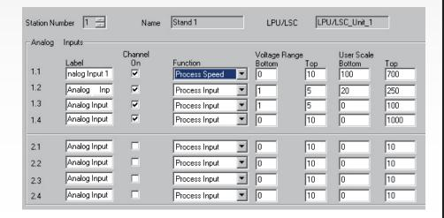
The dialog box shows a system with 8 analog inputs, 4 of which have been activated, the first input was configured for a line speed transmitter scaled 100 to 700 Feet per Minute for a 0-10Volt signal. The next 3 channels are for other process transmitter inputs.
