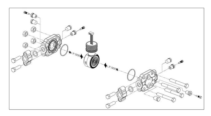
Figure 31 – STG730, 740, 770, and STA722, 740 Transmitter Body (Ref.)
