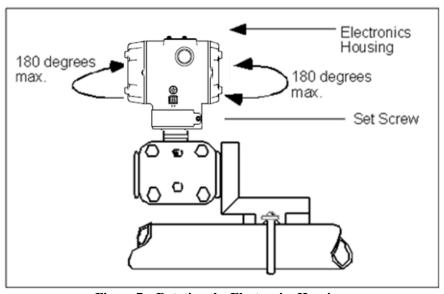
Figure 7 – Rotating the Electronics Housing
