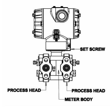
Figure 23 – Hardware Location to Remove the Meter Assembly
