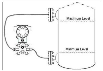
Figure 10 - Representative Remote Diaphragm Seal Transmitter Installation
