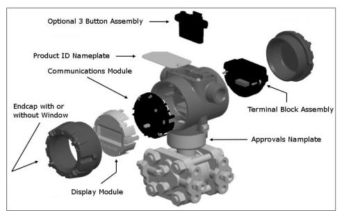
Figure 2 – Electronics Housing Components
