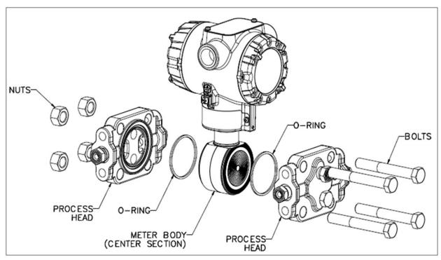
Figure 19 – DP Transmitter Head Disassembly
