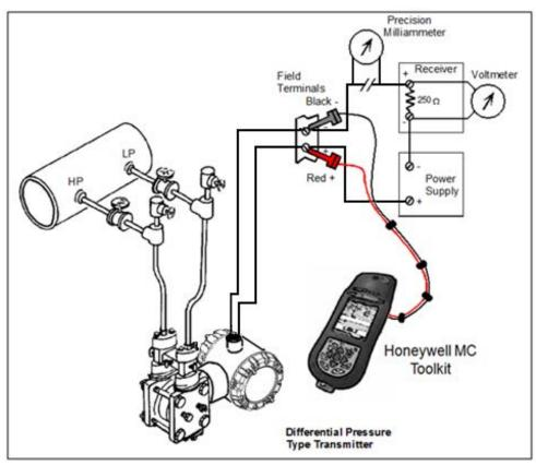
**Figure 15 – Current Loop Test Connections**
