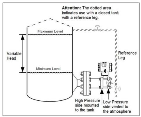
Figure 9 – Tank-Flange Mounted Transmitter
