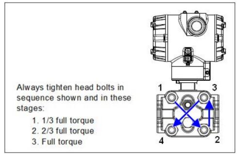
Figure 25 – Head Bolt Tightening Sequence
