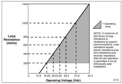
Figure 13 – Transmitter Operating Ranges
