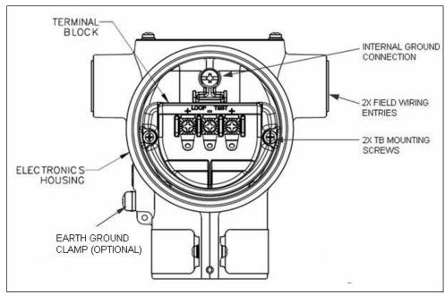
Figure 14 - Transmitter 3-Screw Terminal Board and Grounding Screw
