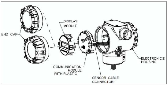
Figure 22 – Disassembly for Meter Body Replacement
