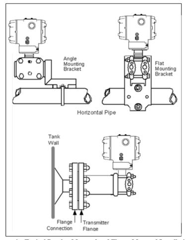
Figure 4 - Typical Bracket Mounted and Flange Mounted Installations
