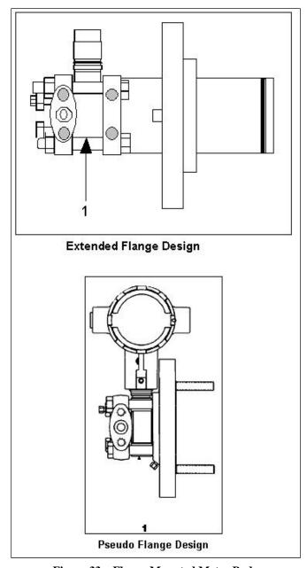
Figure 33 – Flange Mounted Meter Body
