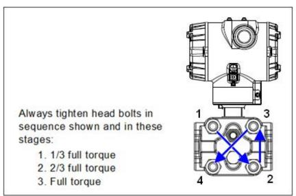
Figure 20 – Head Bolt Tightening Sequence
