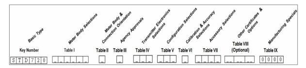
Figure 3 - Typical ST 700 Name Plate
