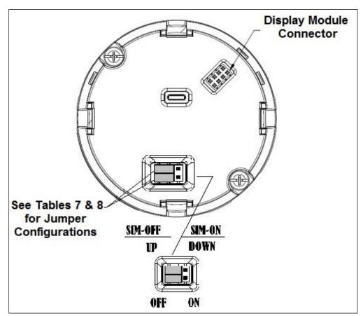
Figure 17 – Locating the Failsafe and Write Protect Jumpesr
