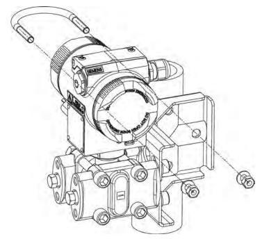
Figure 3-2 An example of fastening the transmitter on the mounting bracket in the case of differential pressure and horizontal differential pressure lines
