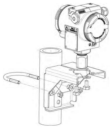
Figure 3-1 Fastening the transmitter on the mounting bracket
