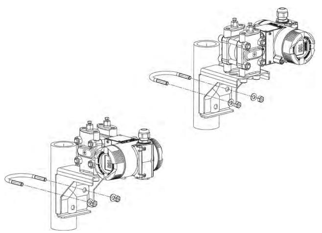
Figure 3-3 An example of fastening on the mounting bracket in the case of differential pressure and vertical differential pressure lines
