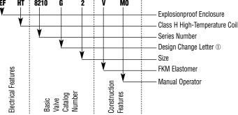
① The Design Change Letter indicates a major design change affecting spare parts kits, rebuild kits, and coils. The correct replacement parts for each change letter are shown in ASCO's Rebuild Kits and Coils Catalog.
