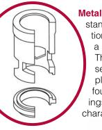
Metal Seated Cage: the standard cage construction is a cast cage with a separable seat ring. The dual function cage serves as a massive plug guide and has four contoured openings to determine flow characteristic.
