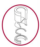
**Soft Seated Cage:** a cast cage with separable seat ring and TFE insert. The soft seat design is used when ANSI Class VI bubble-tight shutoff is desired.
