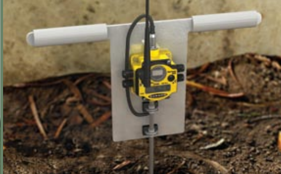
Compost Temperature Monitoring
