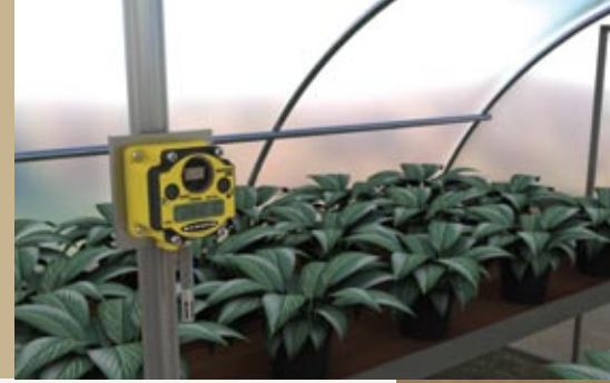
Greenhouse Temperature and Humidity Monitoring
