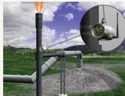
Flare Stack Ignition Verification
