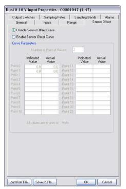
Figure 7.5: Setting a 22-Point Curve Using Wireless Management Toolkit
