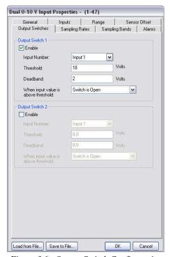
Figure 3.6: Output Switch Configuration Using Wireless Management Toolkit
