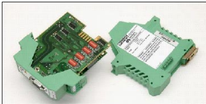
Figure 3. Open the RAD-ISM-900-BD-BUS transceiver to expose the DIP-switches
