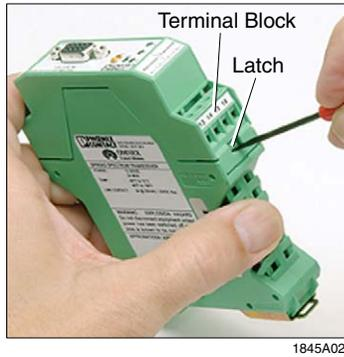
Figure 3-4. Opening Housing to Access DIP Switches
