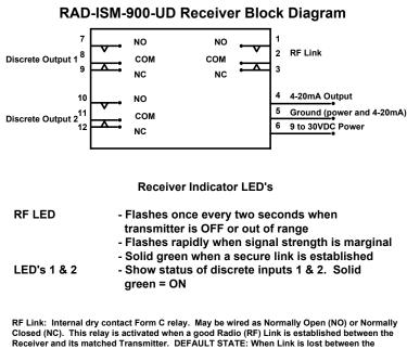
Closed (NC). This relay is activated when a good Radio (RF) Link is established between the Receiver and its matched Transmitter. DEFAULT STATE: When Link is lost between the Transmitter and Receiver, this discrete output defaults to the normal position as shown in the Receiver Block Diagram.
